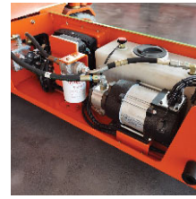
AC Driving Pump Station
